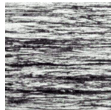
Completely drawn with 89.5 % decrease in cross section
